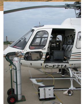
Figure 3. Airborne and ground-based techniques are used in field studies to locate and test legacy wells for methane emissions.
